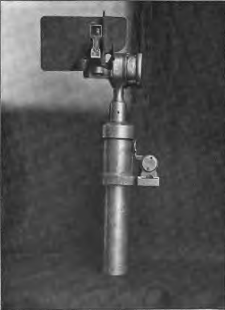
GONIOMETER (FRENCH) FOR TRAINING GUNS IN AZIMUTH.
